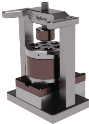
The ASC-A placed inside of the pressure frame.
