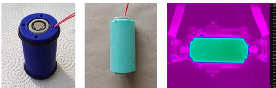
Fig. 2 - Left/Middle: Integration of Pa T100 sensor for temperature monitoring in gap filler encased battery cells. Right: IR-Picture of a cell coated with gap filler material.
