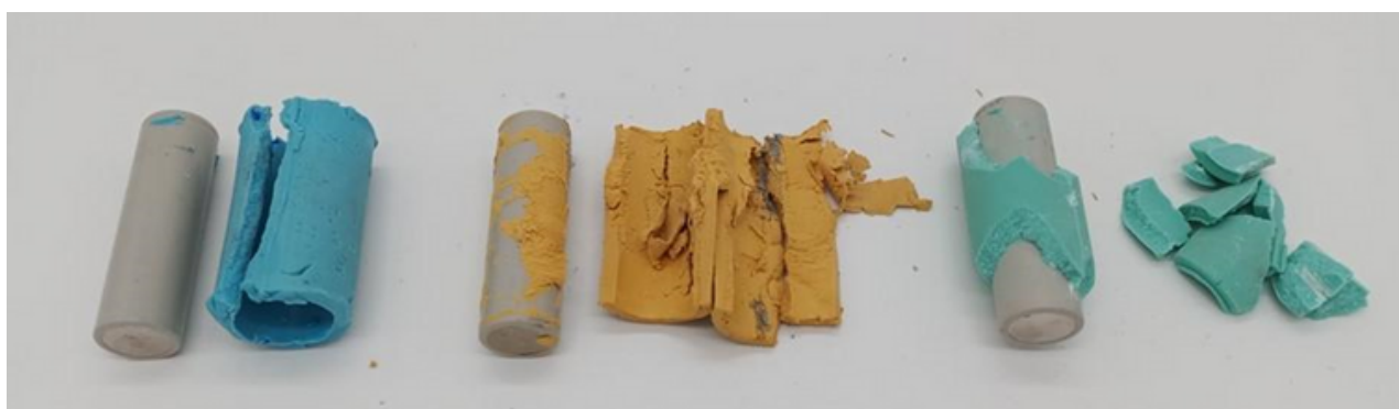
Fig. 5 - The simplicity of the removal of gap filler materials strongly varies among different products. This removal step from battery cells must be considered for 2nd life applications or recycling to reduce processing cost.
